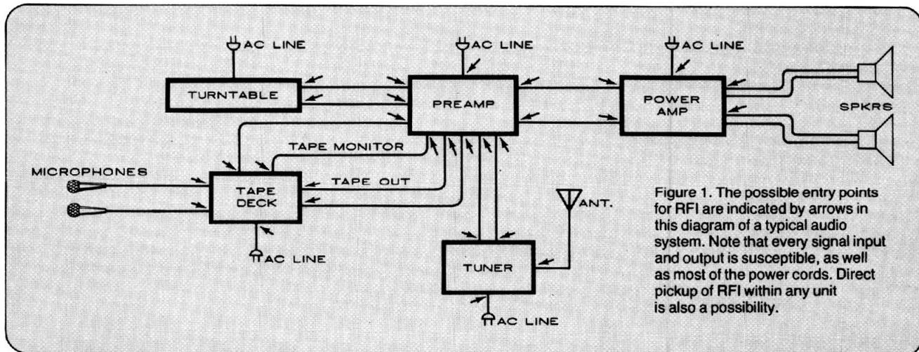
Figure 1. The possible entry points for RFI are indicated by arrows in this diagram of a typical audio system. Note that every signal input and output is susceptible, as well as most of the power cords. Direct pickup of RFI within any unit is also a possibility.
